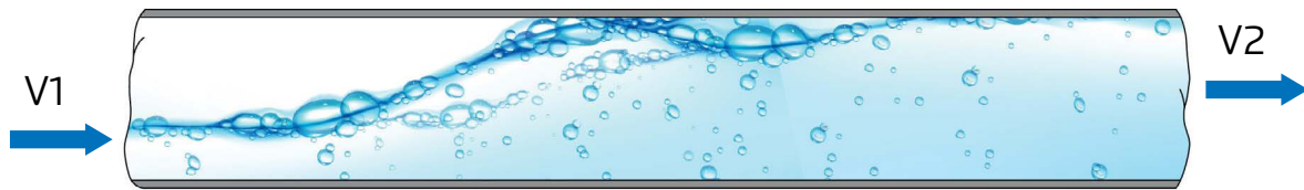
Fig. 31 Air pockets inside the pipe
